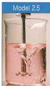
The disperser generates strong vortex motion.
